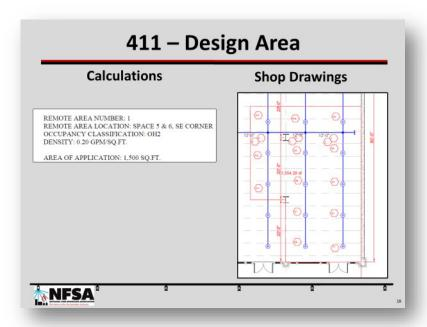
If the project is using the room design method, verify the most remote room, as explained in Step 310 and make a note on the number of design sprinklers. Compare to the requirements for opening protection in Step 311.
