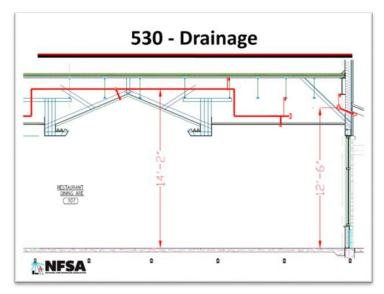
Wet pipe systems are permitted to be installed level. In areas where piping is trapped, an auxiliary drain is required to drain the trapped piping. The capacity of trapped piping in gallons should be stated on the shop drawings. From here, NFPA 13 has specific drainage requirements:
