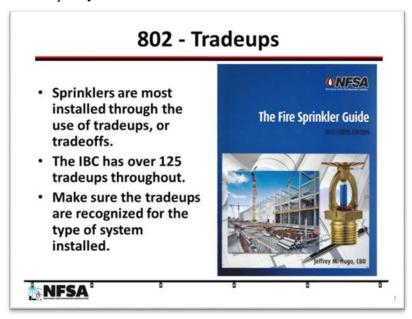
Tradeups do not affect the design or layout of the fire sprinkler system, however the fire sprinkler plans examiner should be aware of the tradeups used to design the building. Tradeups only apply when the building is sprinklered throughout and the fire sprinkler
