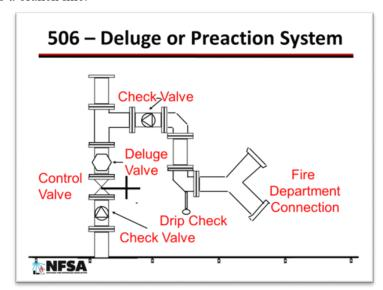
The above figure show where the FDC piping ties into the riser. On systems with multiple risers the FDC piping can be connected anywhere between the system control valves and the supply control valves.
