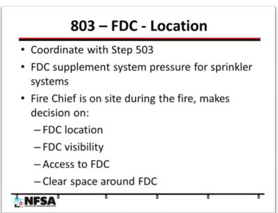
Fire department connections are located and approved by the fire chief. The FDC is to be installed on the street side of the building where it is visible to the responding fire department. The location of the FDC should be such as the fire engine and hose connected to the FDC is not blocking other fire department activities and vice versa. It should be noted that fire hoses are not made to be run over.
