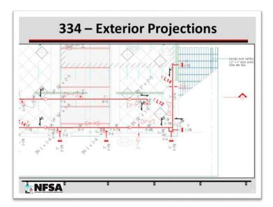
When the exterior projection is combustible, sprinklers are required within the structure and below the structure. However, sprinklers may be exempted from combustible concealed space when filled entirely with noncombustible insulation, when the void space between solid wood joists is firestopped with I-joist material into 160 cubic feet or less, or when the space is less than 55 square feet.
