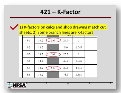
In this step, the plan examiner verifies the sprinkler on the shop drawing correlates with the sprinkler k-factor used in the calculations. Many sprinkler models are available in several k-factors. The hydraulic information (flow, pressure, k-factor) from the cut sheet is verified by the plans examiner to be correctly noted on the worksheet. Accuracy is critical as the k-factor determines the flow and pressure of the sprinklers.
