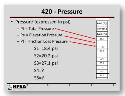
Total pressure  $(P_t)$  is the sum of the pressure in the system up to a node. The elevation pressure  $(P_e)$  and the friction pressure  $(P_f)$  is added together and increases (gets larger) as it gets closer to the water supply. The plans examiner will verify that the increases and decreases along the process are correct. While computer software does the calculations, it is wise to spot check the input in various places.
