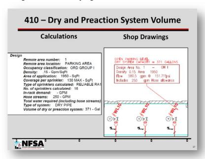
The size of preaction systems varies on the type of system installed. For single and non-interlock preaction systems, the system may not have more than 1,000 sprinklers installed for each preaction valve.
