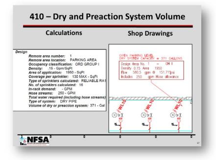
The size of preaction systems varies on the type of system installed. For single and noninterlock preaction systems, the system may not have more than 1,000 sprinklers installed for each preaction valve.
