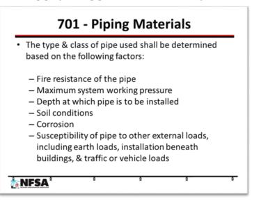
The fire sprinkler plan examiners job is to make sure all the piping, and the joints are acceptable to use, and the shop drawings address the installation requirements.
