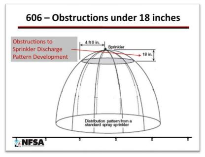
The obstructions rules within 18 inches have unofficial names that are not listed as such in NFPA 13, however they are: The Beam Rule (606-1), The Three Times Rule (606-2), The Four Times Rule (606-3) and The Partition Rule (606-4).
