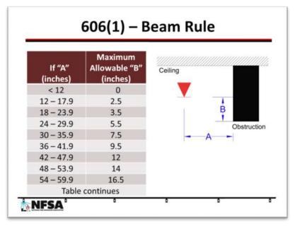
The objective of the Beam Rule is to get the sprinkler far enough away from the near edge of the obstruction that sufficient water will be able to spray under, and beyond, the obstruction. How
