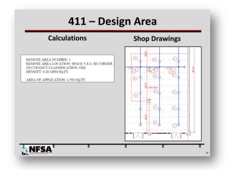
If the project is using the room design method, verify the most remote room, as explained in Step 310 and make a note on the number of design sprinklers. Compare to the requirements for opening protection in Step 311.
