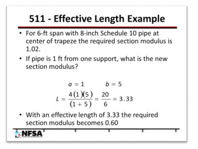
Hangers for ceiling sprinkler system, and trapeze hangers are attached directly to the structural members that are designed. There are a couple exceptions. Pipe of  $1\frac{1}{2}$  inch may be supported by a metal lath or hollow tile ceilings. 1 inch piping may be supported by metal decking. Where piping is installed for in-rack sprinklers protecting storage it is supported by the rack system.
