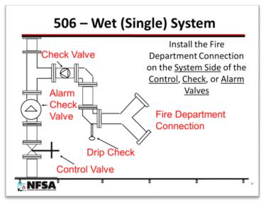
Fire department connection piping is installed on the system side of the check valve. This permits the water that is being pumped into the sprinkler system goes in the right direction. On some systems, there may be other risers and standpipes connected to the FDC. A check valve helps direct flow. This also ensures the water from the fire department pumper tank, which may come from a raw water source, does not go back into the municipal water supply.
