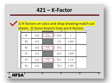
In this step, the plan examiner verifies the sprinkler on the shop drawing correlates with the sprinkler k-factor used in the calculations. Many sprinkler models are available in several k-factors. The hydraulic information (flow, pressure, k-factor) from the cut sheet is verified by the plans examiner to be correctly noted on the worksheet. Accuracy is critical as the k-factor determines the flow and pressure of the sprinklers.
