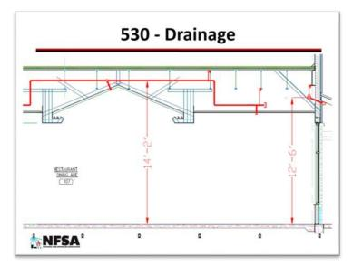
Wet pipe systems are permitted to be installed level. In areas where piping is trapped, an auxiliary drain is required to drain the trapped piping. The capacity of trapped piping in gallons should be stated on the shop drawings. From here, NFPA 13 has specific drainage requirements:
