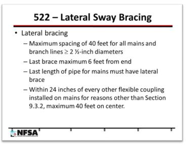
Lateral bracing is not required where U-type hooks have legs bent to a minimum 30degree angle and the lengths comply with Tables 9.3.5.11.8(a)-(c). Lateral bracing is also not required when the distance from the top of the pipe and the bottom of the structure is less than 6 inches.
