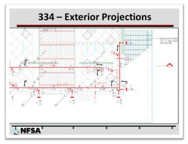
When the exterior projection is combustible, sprinklers are required within the structure and below the structure. However, sprinklers may be exempted from combustible concealed space when filled entirely with noncombustible insulation, when the void space between solid wood joists is firestopped with I-joist material into 160 cubic feet or less, or when the space is less than 55 square feet.
