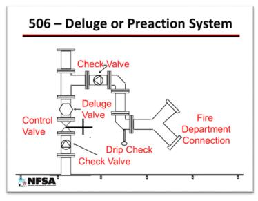
The above figure show where the FDC piping ties into the riser. On systems with multiple risers the FDC piping can be connected anywhere between the system control valves and the supply control valves.
