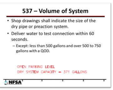
Dry pipe systems are required to deliver water to the test connection within 60 seconds. This rule does not apply to systems that are 500 gallons or less or for systems that are 750 gallons or less when equipped with a quick-opening device.
