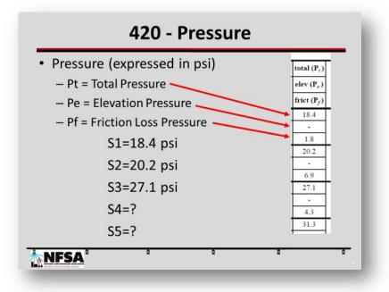
Total pressure  $(P_t)$  is the sum of the pressure in the system up to a node. The elevation pressure  $(P_e)$  and the friction pressure  $(P_f)$  is added together and increases (gets larger) as it gets closer to the water supply. The plans examiner will verify that the increases and decreases along the process are correct. While computer software does the calculations, it is wise to spot check the input in various places.
